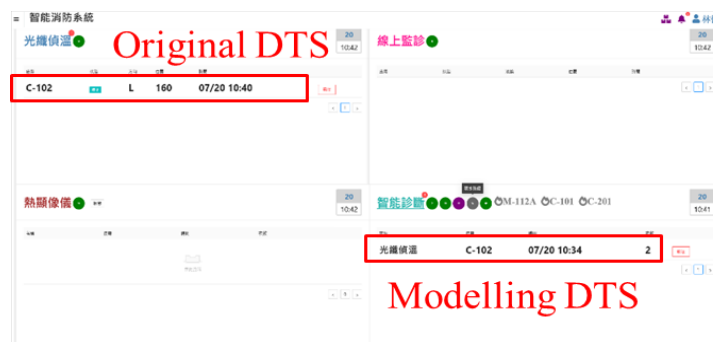
Fig.11. The System display of HMI (Modelling DTS alert 6 minutes earlier than Original DTS).
