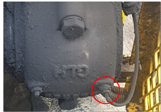
Fig.5. The deployment of thermocouple for BTS.
