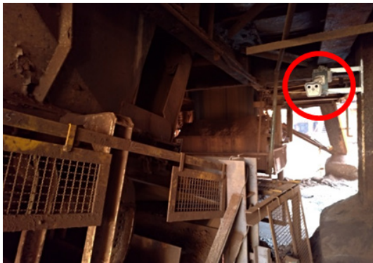
Fig.7. The deployment of thermal camera.
