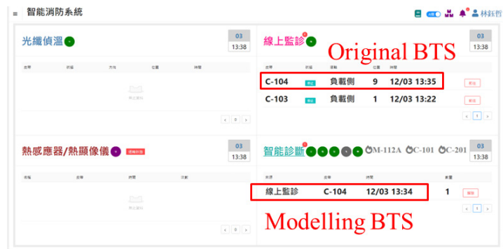
Fig.14. The System display of HMI (Modelling BTS alert 1 minutes earlier than Original BTS).
